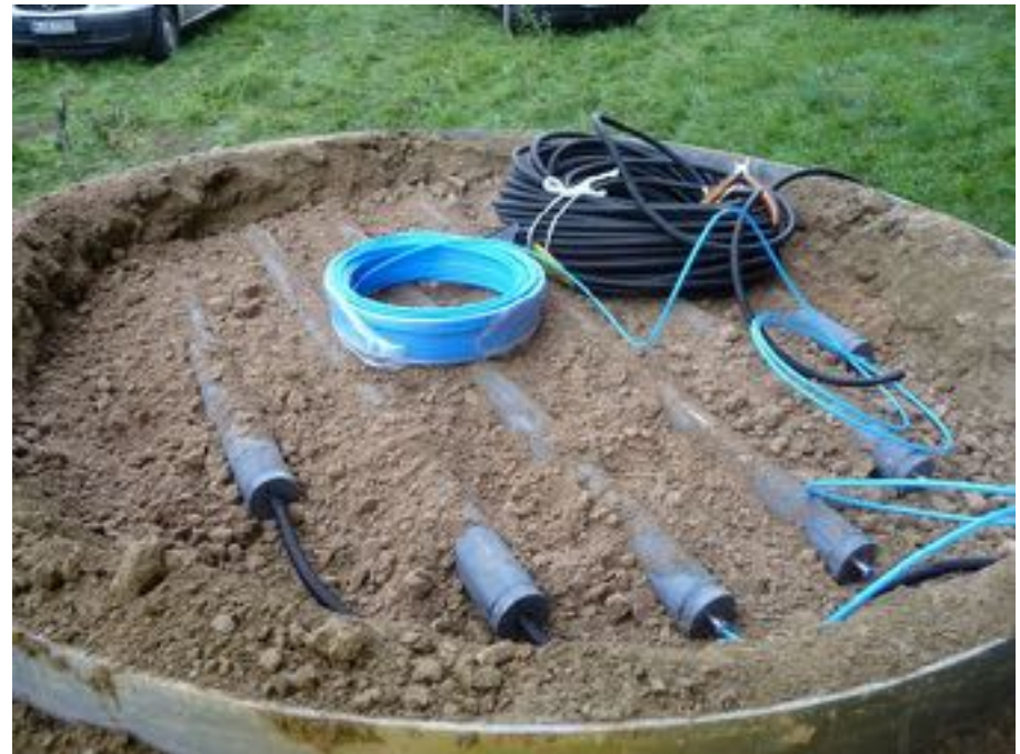
Suction cups rack for lower boundary condition
